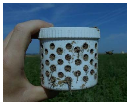
Figure 1: Schematic representation of a pot and plate trap as well as an image of a Meles pot trap (Photo: Meles GmbH, www.melesbio.at ).
