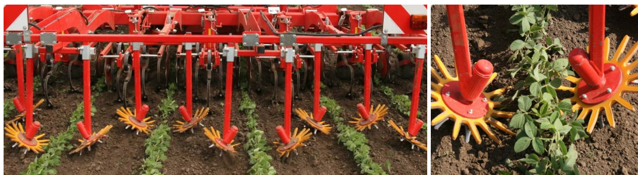
Picture 1: Combination of finger weeder and duck-foot tines in soy. Picture 2: Finger weeder at work within the row. (Pictures: Goran Malidza, Institute of Field and Vegetable Crops, Novi Sad).
