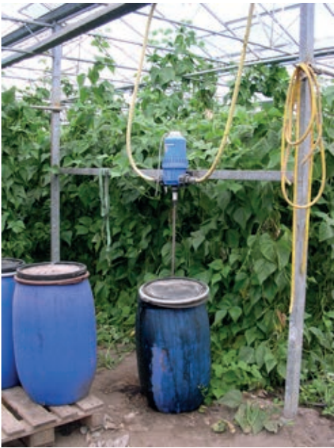
Figure 3.3 Equipment used for fertigation of greenhouse crops, mixing nutrients into the irrigation water.
