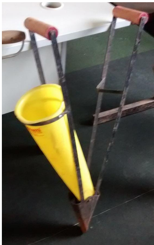
FIGURE 5. The planter open the slot in the soil and to release the seedling.
