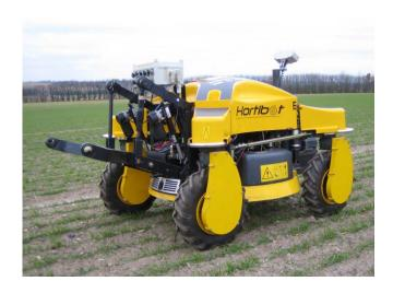
Figure 2. Hortibot field robot
