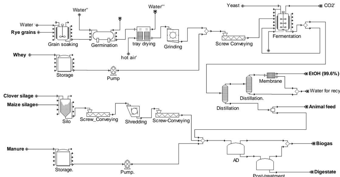
Figure 2. Simplified flow diagram of the organic farm scale biorefinery for the co-production of biogas and bioethanol
