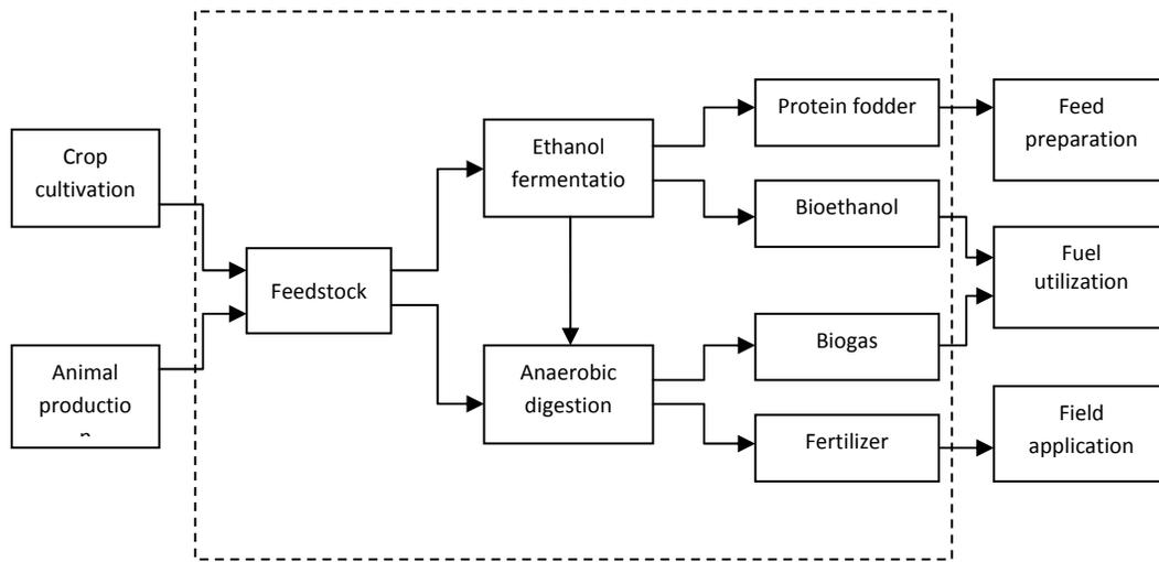
Figure 1. Simplified diagram of the process: The two fuels (bioethanol and biogas) are produced from selected raw materials.
