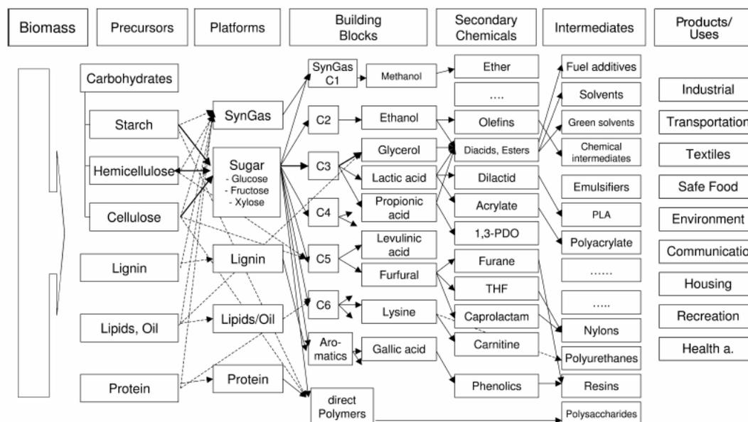
Figure 17. Model of a biobased products flow-chart for biomass feedstock (Werpy and Petersen, 2004)
