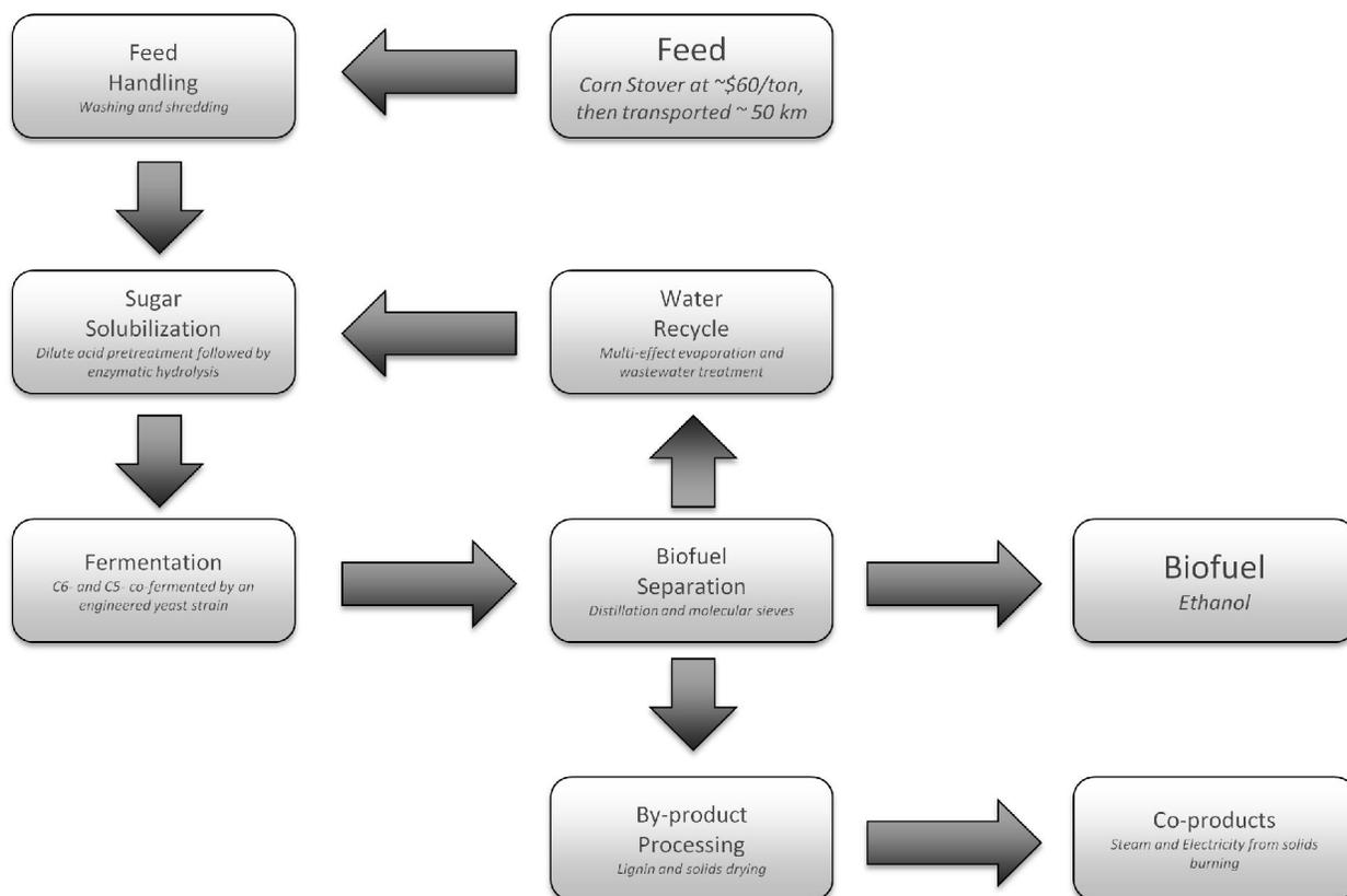
Supplementary Figure 1. General schematic of the lignocellulosic ethanol biorefinery
