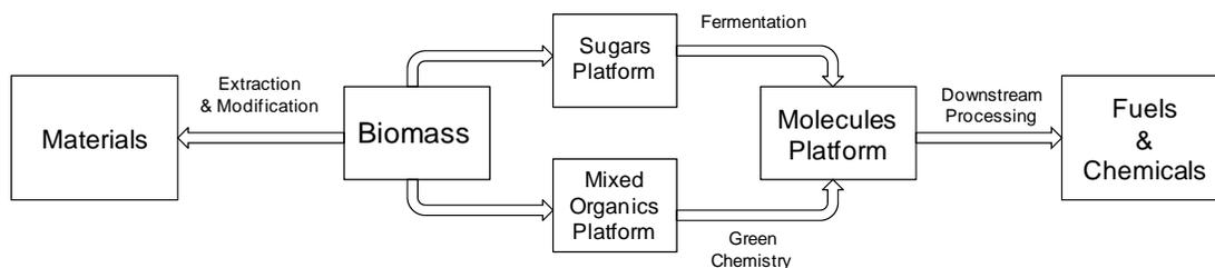
Figure 16. Biorefinery (adapted from Clark, 2007)
