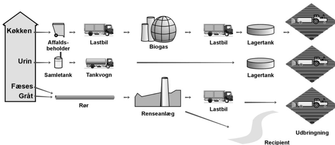
System 2: Kitchen waste is treated in a biogas plant. Urine is collected separately, faeces and grey water are treated on a wastewater plant.
