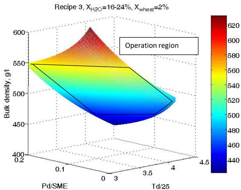
Figure 6 Fish feed extrusion processing simulation results (twin-screw extruder) at  $X_{H_2O}=16-24\%$ ,
