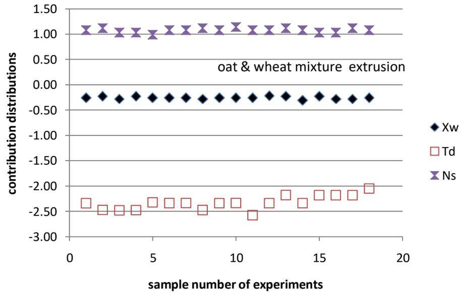
Figure 7 Effects of operation parameters on bulk density, oat & wheat mixture extrusion (single-screw extruder).  $\blacklozenge$  Xw is the  $\alpha \ln X_w$ ,  $\square$  Td is the  $\beta \ln \left(\frac{T_d}{T_0}\right)$ ,  $\times$  Ns is the  $-\gamma \ln(N_s)$  in equation(7)
