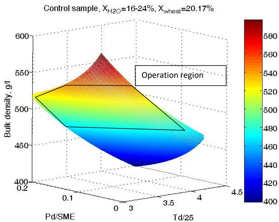
Figure 5 Fish feed extrusion processing simulation results (twin-screw extruder) at  $X_{H_2O}=16-24\%$ ,  $X_{wheat}=20.17\%$ , control recipe
