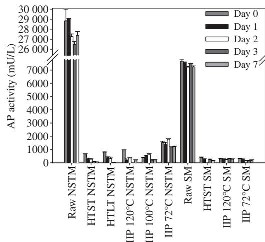
**Figure 3** Experiments 4a and 4b. Effect of storage time of 0–7 days at 5°C of nonstandardised (NSTM) milk and skim milk (SM) samples on alkaline phosphatase (AP) activity for selected treatments of Raw = unprocessed, IIP = instant infusion pasteurised, HTST = high temperature short time in plate heat exchange (72°C/15 s) and HTLT = high temperature long time in plate heat exchange (85°C/30 s),  $n = 3$ .
