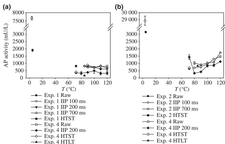
**Figure 2** Alkaline phosphatase (AP) activity as function of treatment temperature  $T$  for (a) skim milk Experiments 1 and 4a, and (b) nonstandardised milk Experiments 2 and 4b, as Raw = unprocessed, IIP = instant infusion pasteurised at the given holding times from 100 to 700 ms, HTST = high temperature short time in plate heat exchange ( $72^{\circ}\text{C}/15$  s) and HTLT = high temperature long time in plate heat exchange ( $85^{\circ}\text{C}/30$  s),  $n = 3$ .
