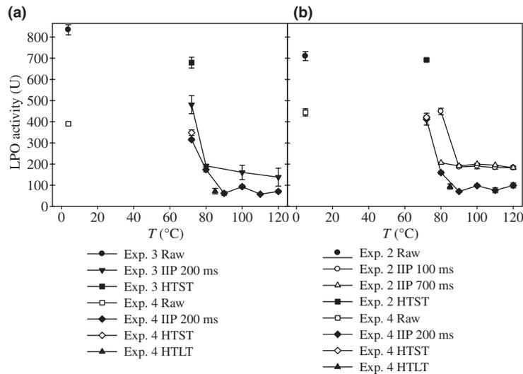
**Figure 4** Lactoperoxidase (LPO) activity as function of treatment temperature  $T$  for (a) skim milk Experiments 3 and 4a and (b) NSTM Experiments 2 and 4b, as Raw = unprocessed, IIP = instant infusion pasteurised at the given holding times from 100 to 700 ms, HTST = high temperature short time in plate heat exchange (72°C/15 s) and HTLT = high temperature long time in plate heat exchange (85°C/30 s),  $n = 3$ .
