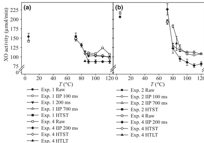
**Figure 5** Xanthine oxidase (XO) activity as function of treatment temperature  $T$  for (a) skim milk Experiments 1 and 4a and (b) nonstandardised milk Experiments 2 and 4b, as Raw = unprocessed, IIP = instant infusion pasteurised at the given holding times from 100 to 700 ms, HTST = high temperature short time in plate heat exchange (72°C/15 s), and HTLT = high temperature long time in plate heat exchange (85°C/30 s),  $n = 3$ .
