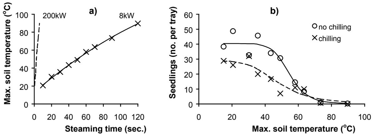
Figure 2. a): measured (x) and modelled (—) relationship between achieved maximum soil temperature and steaming time with 8 kW effect and the same theoretical relationship with 200 kW effect (---). b): relationships between number of emerged seedlings (weed plus crop seeds) and maximum soil temperature with (---) or without (—) chilling.
