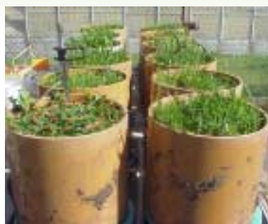
Injection of ^{15}N -labelled NH_4 and NO_3 (10 APE) in 30 cm diam. x 25 cm high monoliths of the grass-clover pastures.
