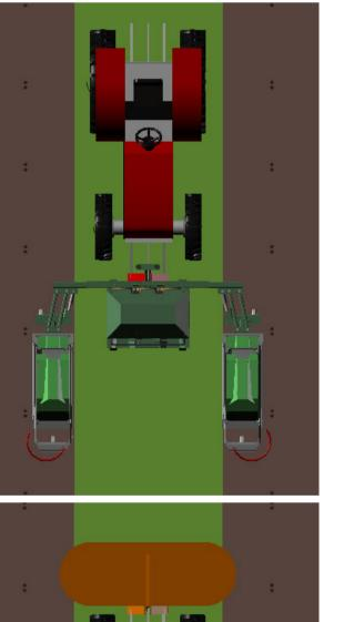
**Orchard Tractor** 2 burners placed at the back. **Combined with** Lawnmover
