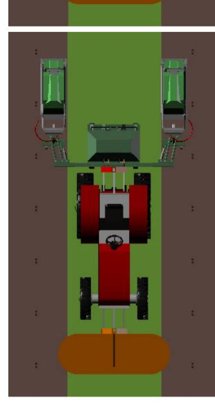
The modular burner system for burning weeds in orchards can be configurated to your needs. You can also choose to build it with a lawnmower and thereby save time.
