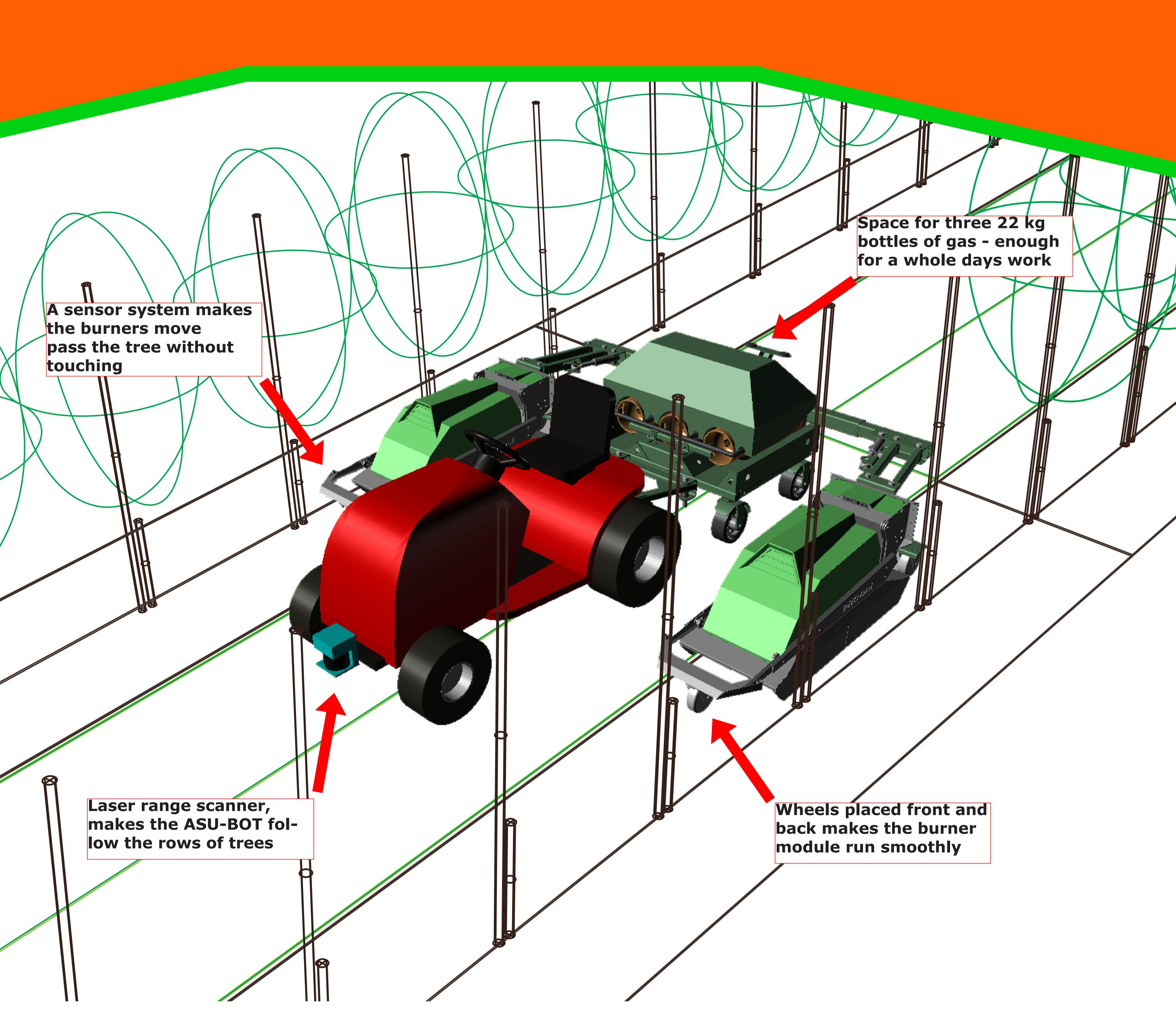
Gas burning makes treatment of weed organic. The new ENVO-DAN burner saves 40% gas and treats ½ meter in width. It can be mounted on a standard lawn tractor, orchard tractor or a mobile robot.
