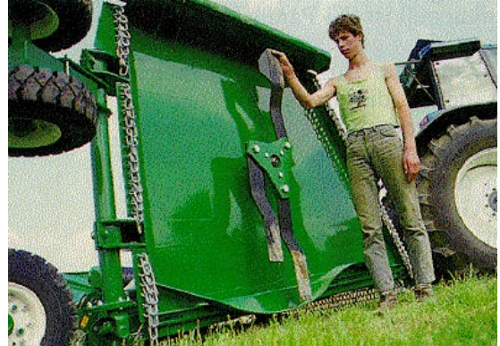
Figure 8: Cutter-assembly of rotary mulching machine (dlz. 2/1997. n.80)
