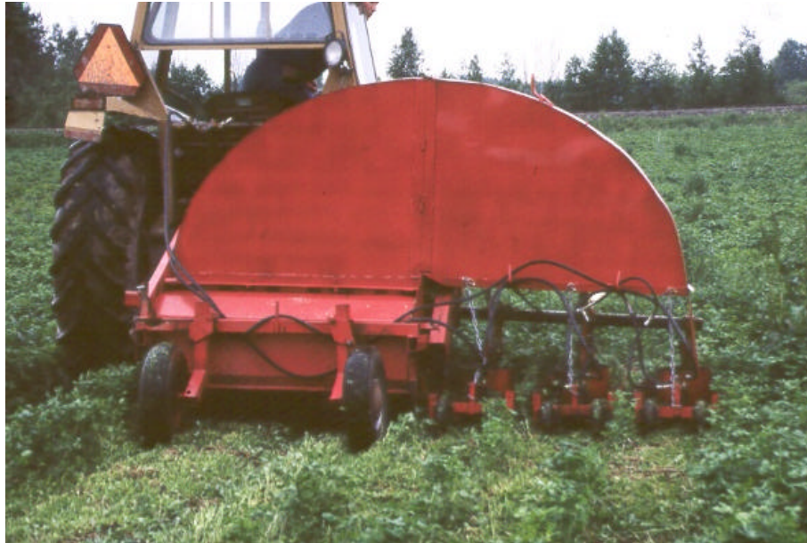
Figure 23: Prototype of the green mulch spreading-machine of Agricultural Engineering Research Unit
