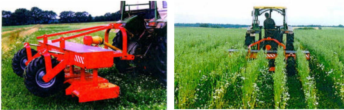
Figure 18: Row-mulching machine (Helmut Fischer Ltd., Gemmrigheim, Germany)
