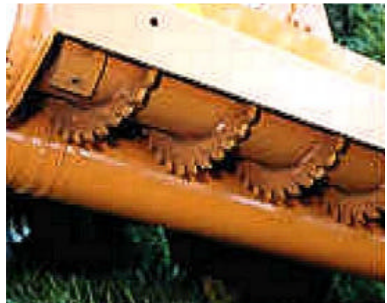
Figure 10: Toothed screw-mulching tool (Maschinenfabrik Bermatingen GmbH&Co., Germany)
