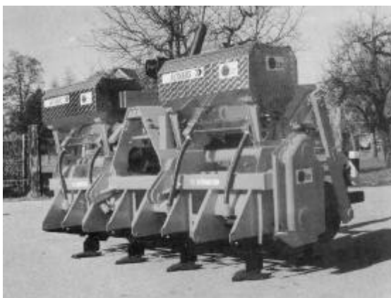
Figure 19: Strip rotary tiller with direct seed device. (Althaus Co. AG, Ersingen, Swiss)
