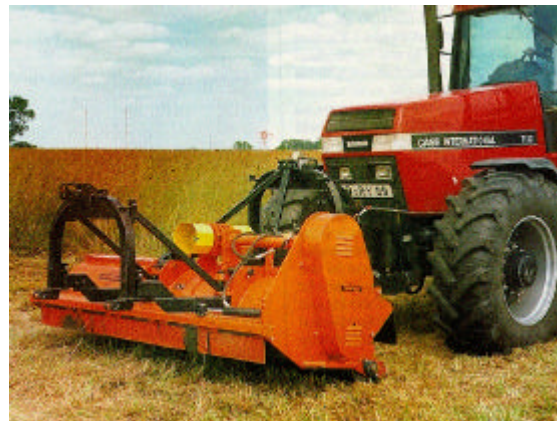
Figure 6: Front mounted flail mulching machine (HASS 1996)
