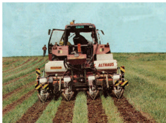
Figure 20: Multipurpose strip rotary and direct seed machine (ANONYM 1993)
