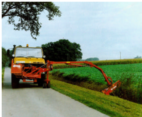
Figure 11: Roadside mulcher (Gerhard Düker KG, Germany)
