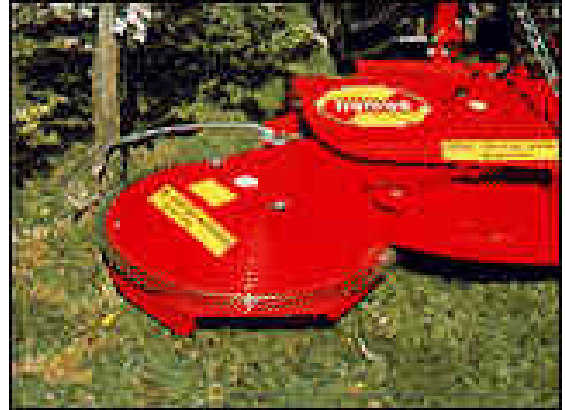
Figure 15: Sensor operated swivel arm mulcher (Maschinenfabrik Bermatingen GmbH, Germany)
