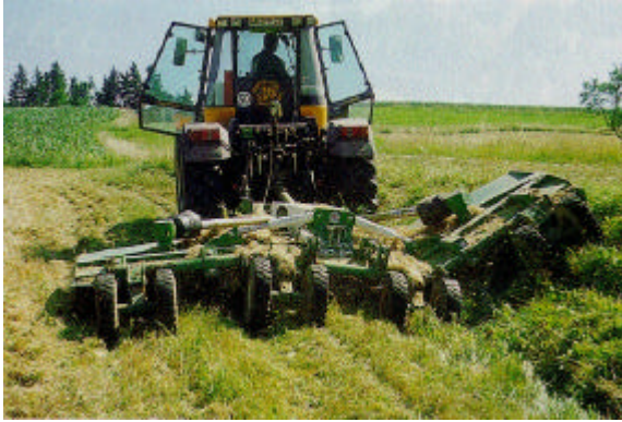
Figure 7: Rotary mulching machine (dlz, 2/1997, p.80)
