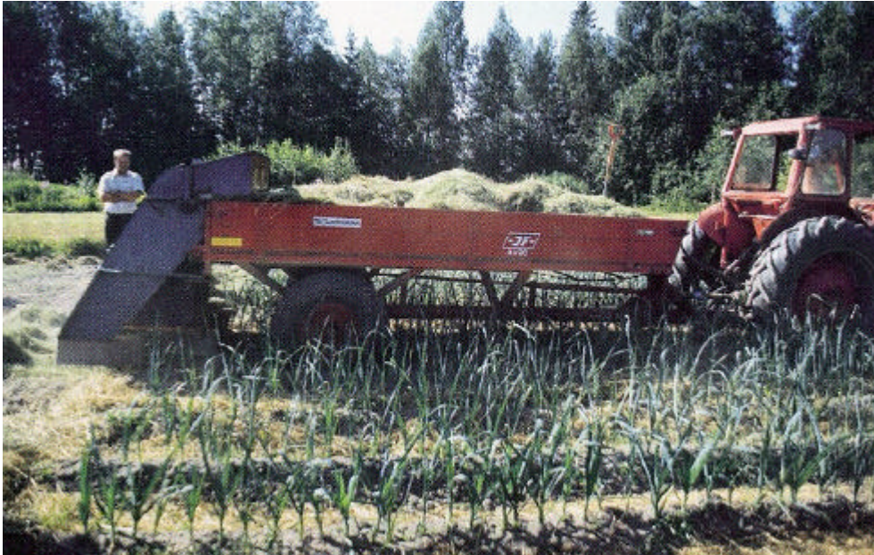
Figure 26: Technique A, modified manure spreader (Luomulehti 7/97)
