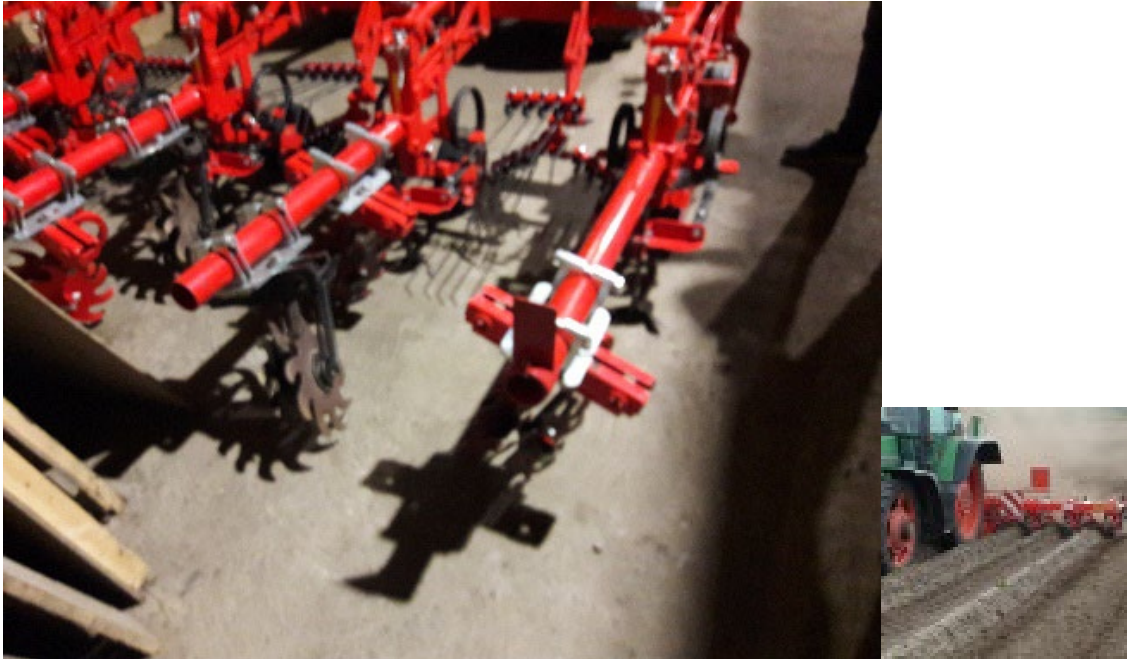
Einböck ridge band cultivator with inclined mounted star wheels is used for weeding.
