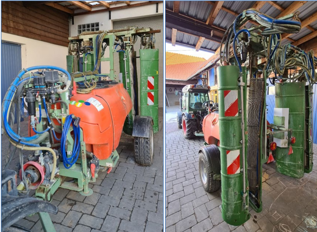
Figure 1. Special sprayer with equipment for collecting and recycling of excess spraying liquid.
