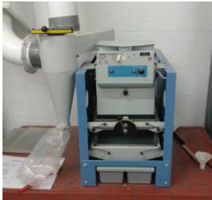
**Sample cleaner** to remove debris from seed material. [Photo: CS]
