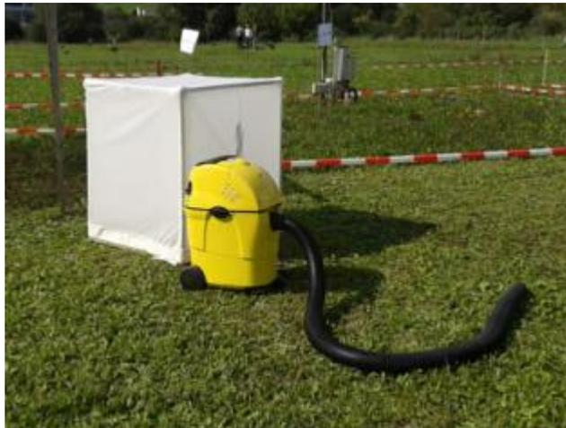
**Biocoenometer (suction sampler).** Allows volume-specific sampling but is rather labour-intensive. [Images: CS]
