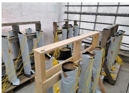
**Figure 3** Root observation-pots (24) attached to wooden pallets for support. The white plastic film is wrapped around the pots to prevent light exposure to the soil.
