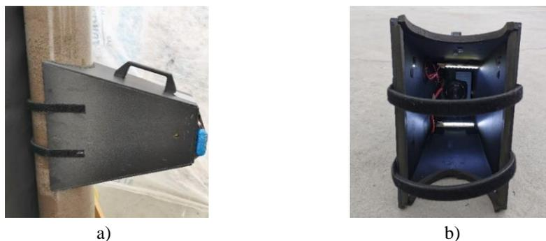
**Figure 6** The PhotoBox used for obtaining root images from the pot-soil interface as seen from a) the side view and the b) front view where the lens and the LED lights are shown.
