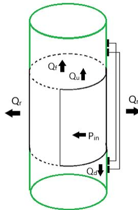
**Figure 1** An annular heater on a stem section and heat fluxes of the heat balance theory. A constant and steady state energy input is applied ( $P_{in}$ ) to the stem section which results in heat fluxes radially to the ambient ( $Q_r$ ), vertically in the stem ( $Q_u, Q_d$ ) and the one carried by the sap flow ( $Q_f$ ).
