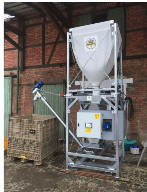
Photo 1: Toasting technology treats soya beans with steam or hot air. Photo: EST GmbH
