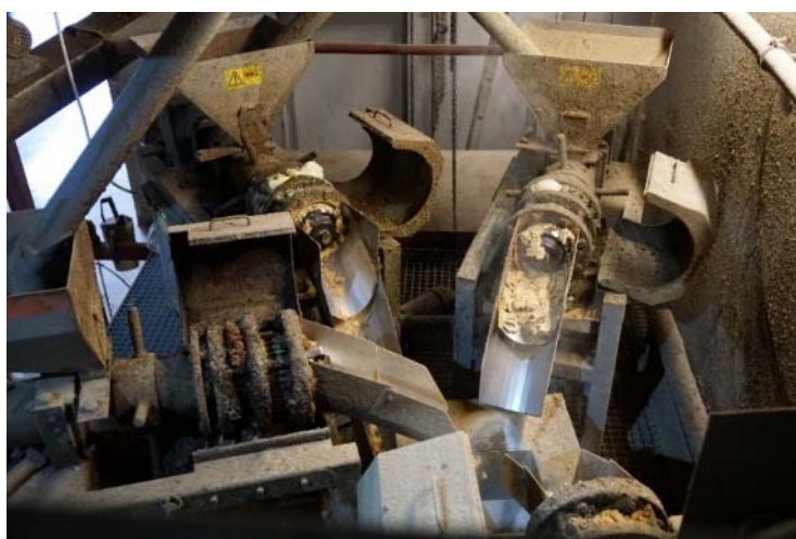
Photo 4: Oil presses are common in soya bean processing. In this case, four presses are combined. Photo: Donau Soja
