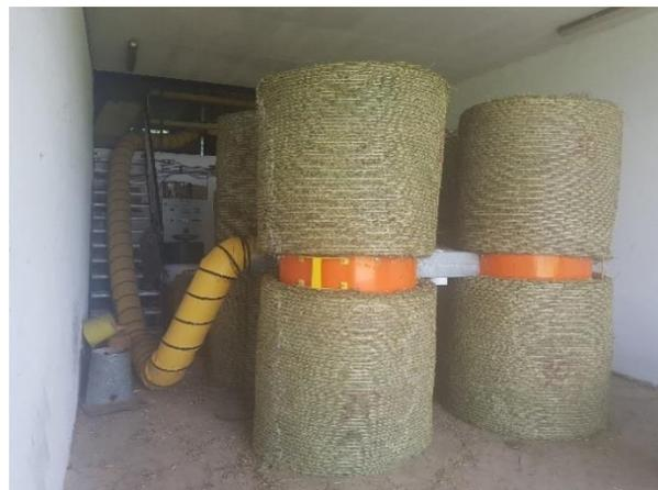
**Figure 6: Ventilation of bales.** Photo: Anton Elsasser
