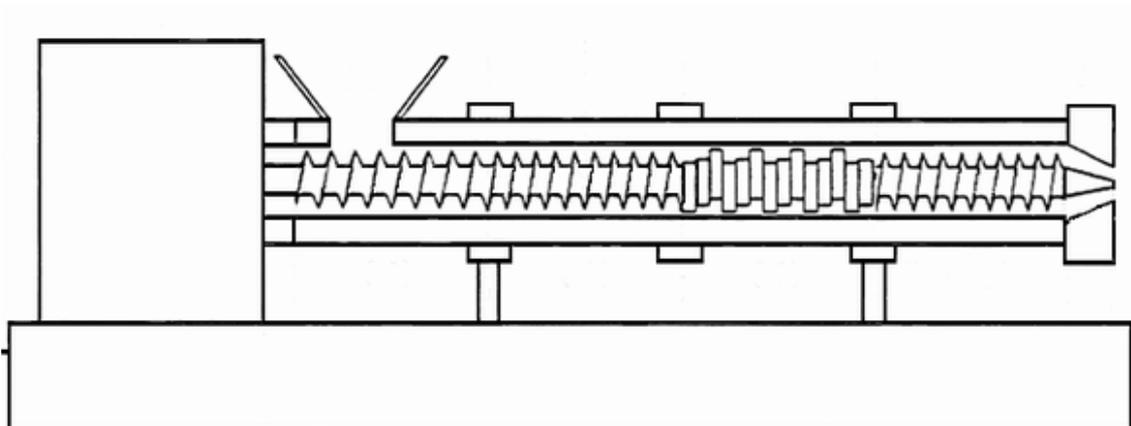
Figure 3 Single screw extruder. (Mehuys 2004)
