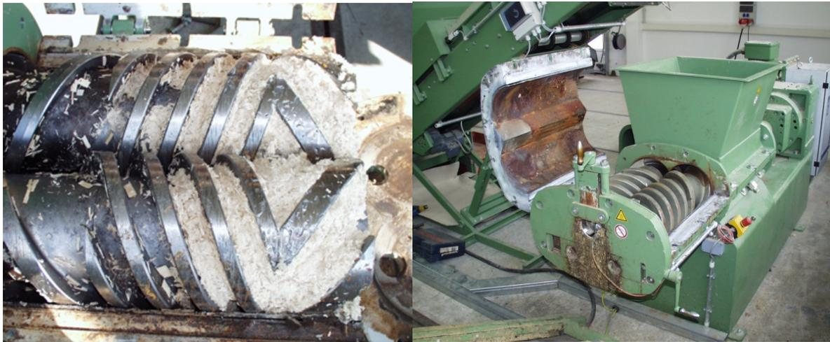
Figure 2. Open twin screw extruder with material inside (left), whole extruder opened (right).
