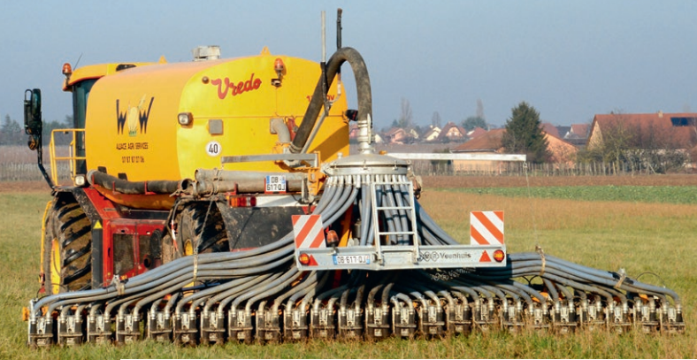
Due to their high ammonium contents, liquid digestates should be applied to N demanding crops using special devices to avoid major ammonia losses.
