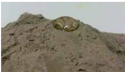
Figure 2. Water droplet on hydrophobic soil.
