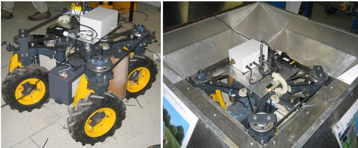
Figure 2. Left – The remotely controlled mobile unit. Right – The remotely controlled mobile unit within the pyramidal feeder construction (see also figure 3 right)
