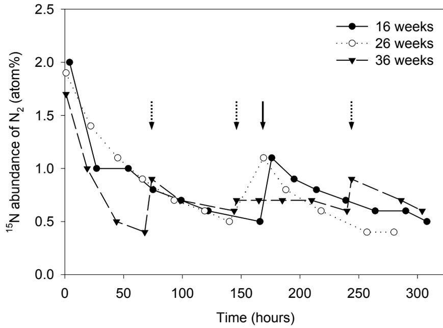
Figure 2. Changes in  $^{15}\text{N}$  abundance of atmospheric  $\text{N}_2$  in the labelling cabinet during the incubation at 16, 26 and 36 weeks after plant emergence. Arrows indicate time for additional  $^{15}\text{N}_2$  supply (solid arrow = 16 and 26 weeks, dashed arrows = 36 weeks).
