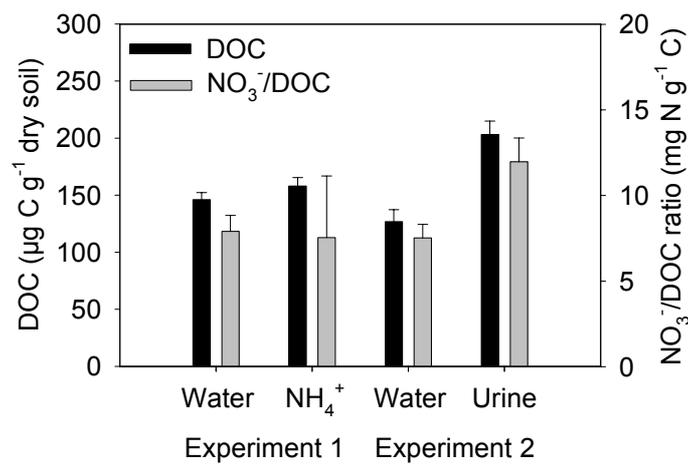
Figure 2. Soil content of dissolved organic carbon (DOC) and the  $\text{NO}_3^-/\text{DOC}$  ratio in the 0-10 cm soil layer of microplots treated with water, ammonium solution and urine;  $n = 4$ ; means  $\pm$  SE.
