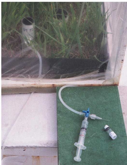
Figure 6. Equipment for measurement of gas emission from grassland monolith placed in a  $^{13}\text{C}$ -labelling facility.
