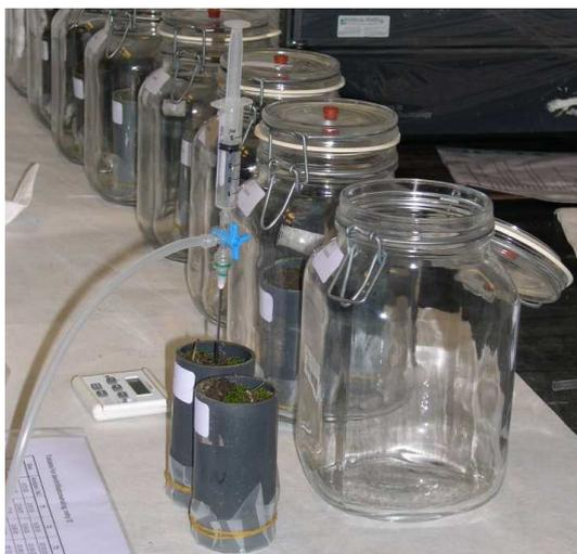
Figure 8. Injection of acetylene into a soil core prior to incubation in a glass jar.
