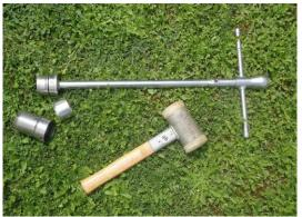
Figure 2. Hammer-driven double-cylinder sampler
