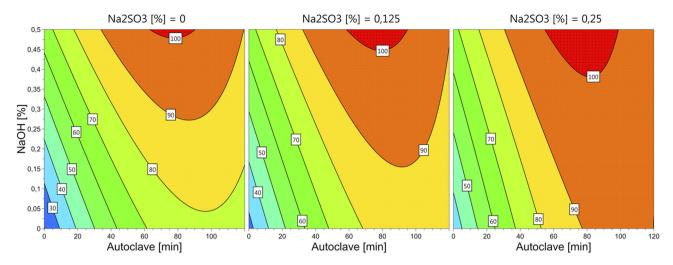
Figure 3. Contour plot for total in vitro pepsin digestibility (solubilized and residual fractions combined) (%) of chicken feather hydrolysates as affected by concentrations of NaOH, Na<sub>2</sub>SO<sub>3</sub> and autoclaving time.
