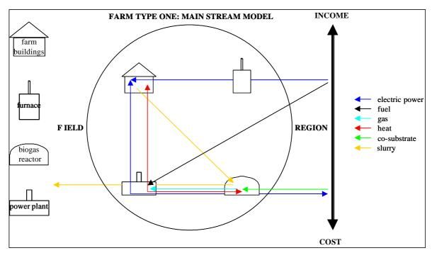
biogas powers a diesel engine of 26 kW electric power capacity using 10% ignition diesel fuel. Electric power production covers 70% of farm consumption and a surplus that amounts to 84% of the production is supplied to the main grid. Heat energy is used as process energy of the biogas reactor and for heating the farm estate. The surplus amounting to 72% remains unused.
