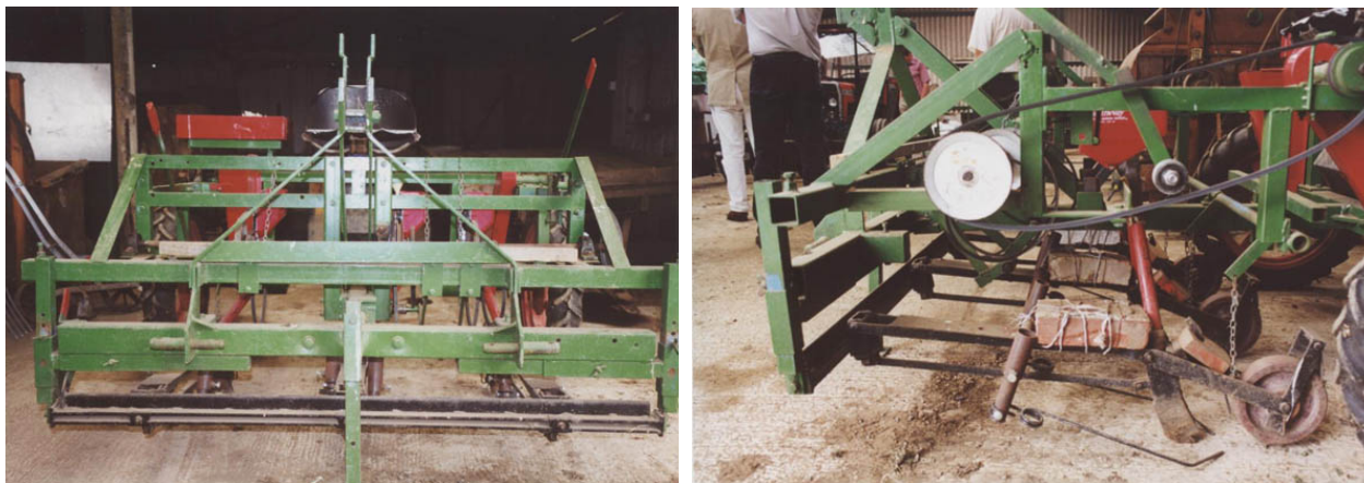
Plate 6. Front and profile view of the seed drill
