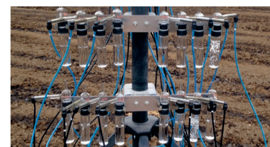
Fig.3 Quantification of NH 3 -emissions via automatized "Low cost impinger system (LOCI)". [5]
