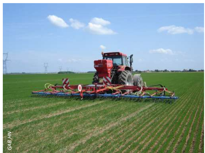
Tine harrow mounted on a seed drill in a linseed field
