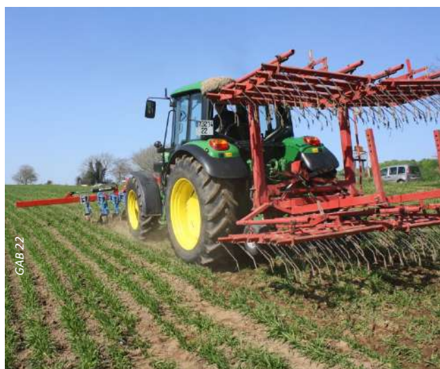
Tine harrow with a front-mounted row cultivator
