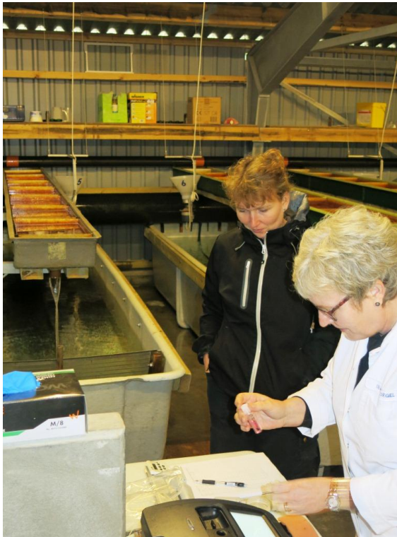
Fig. 3. Spectrophotometric analyses of peracetic acid concentration measured on location, here a commercial Danish hatchery.
