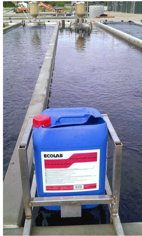
Fig. 1. A practical solution to add PAA over a prolonged period of time. An amount of PAA product diluted in water is added to the farm unit during 1-1½ hours. This ensures a fairly even addition and avoids severe local peak PAA concentrations and drop in pH.
