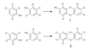
Figure 2. Examples of the formation of (hexachlorodibenzo-p-)dioxins by dimerization of tetrachlorophenol.
